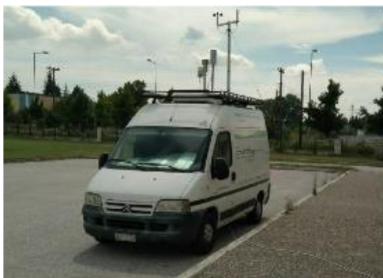
Figure 16 Mobile air quality monitoring station at Thessaloniki (SKG) airport
