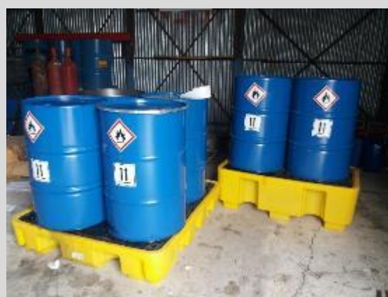
Figure 20: Barrels for used oils stored indoors. The used oils are sent for recycling to the respective Alternative Management System.
